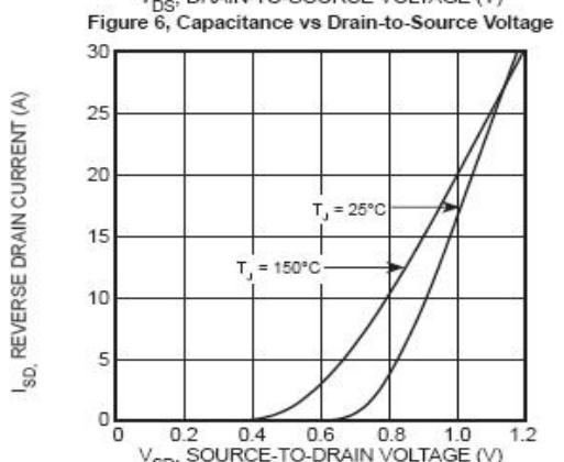
Figure 8, Reverse Drain Current vs Source-to-Drain Voltage
