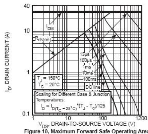
Figure 10, Maximum Forward Safe Operating Area
